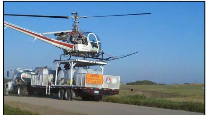
Landing pad and reloading & refueling deck
